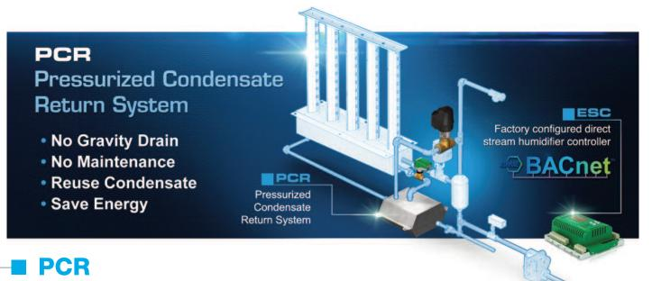
The Neptronic pressurized condensate return (PCR) system returns condensate generated within the steam dispersion tubes of a direct steam humidifier back to the steam source. Presently, the only other available technology is a pressurized steam humidifier with a heat exchanger (or re-evaporator).
