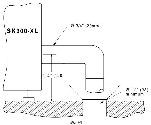
**Enclosure** Water Drain Valve
