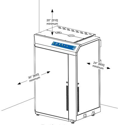
(Fig. 5) Standard enclosure dimensions in bracket are in mm
