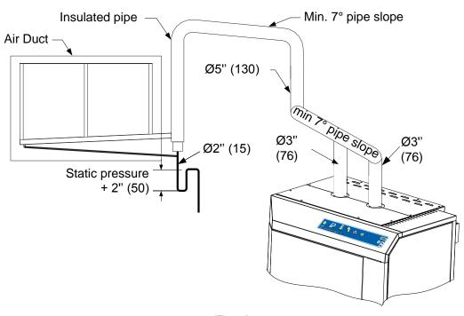
(Fig. 12) dimensions in bracket are in mm
