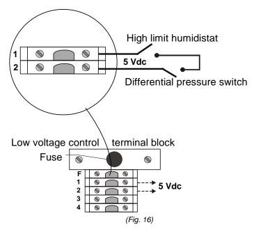
**High level humidistat** contact must be wired in series with **P.D. Switch** contact and humidistat signal between terminals TB1 & 2
