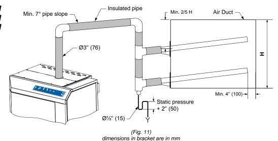
A single Ø3" (76mm) feed pipe must be connected to a single Multi-Steam with a suitable reduction at the lowest point to allow a  $\emptyset^{1/2}$ " (15mm) condensate drain from the main steam supply.
