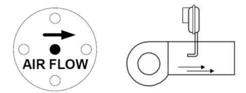
Verify velocity at minimum 300 FPM to activate the heater. Note that certain modulating heaters will have electronic airflow sensors (EAS) built-in, instead of mechanical airflow switches, which do not require any field work.
