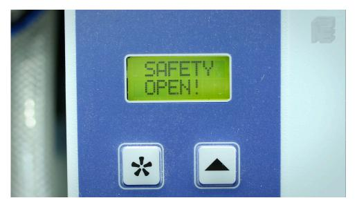
A: "Safety Open" refers to the controls that are wired between the low voltage terminals 1 and 2. It indicates that one of the controls has an open contact.
