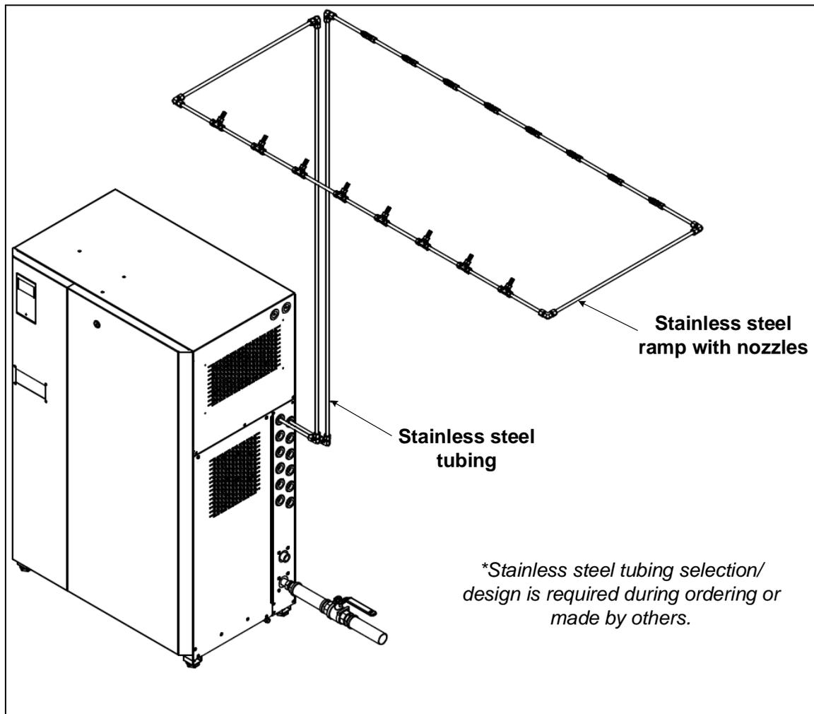
Illustration 18 - Typical Installation with Rigid Nozzle Ramp
