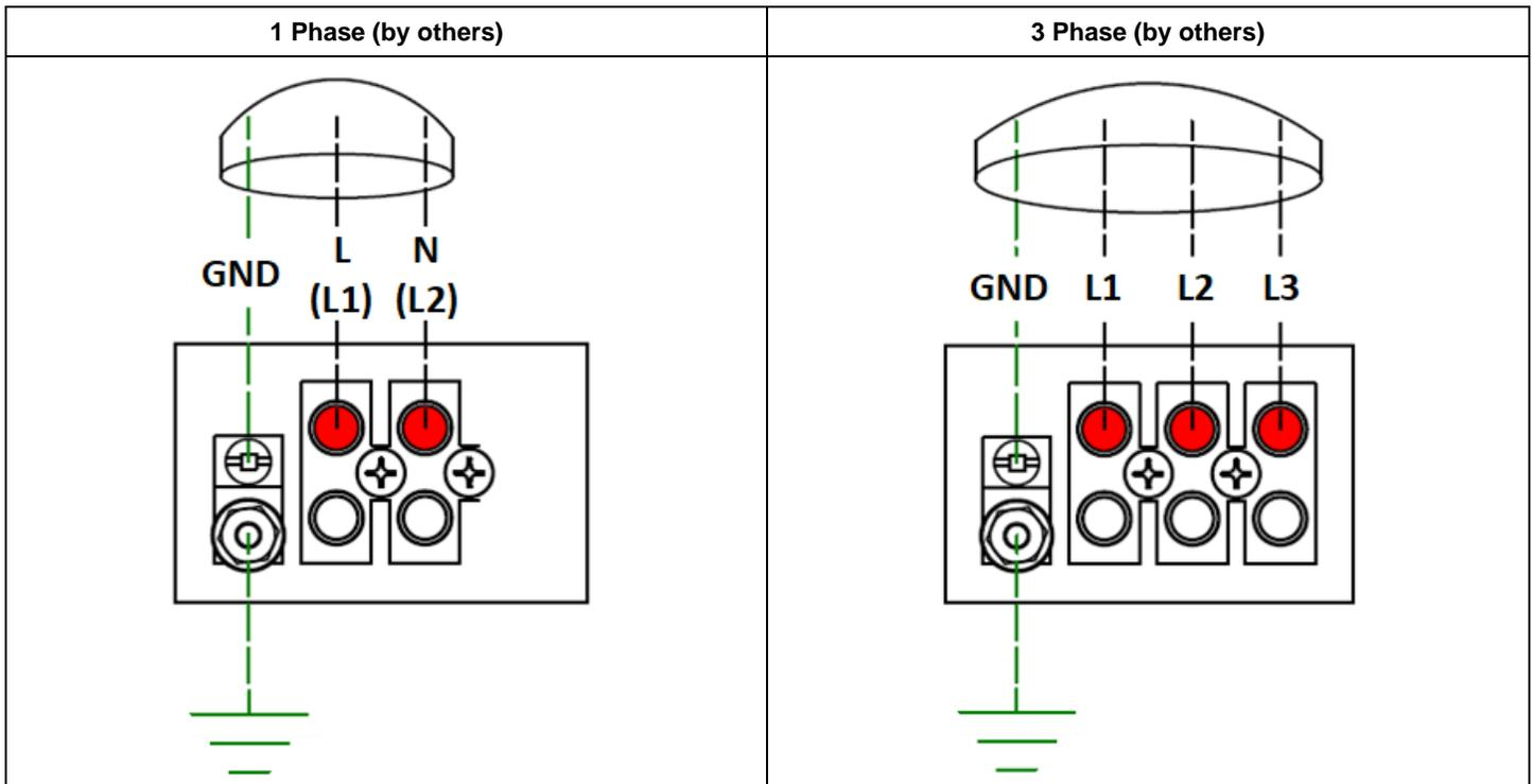
Illustration 11 - One and Three Phase Power Supply Connections
