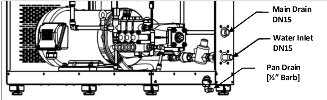
Illustration 9 - Water Connections for Pump Station
