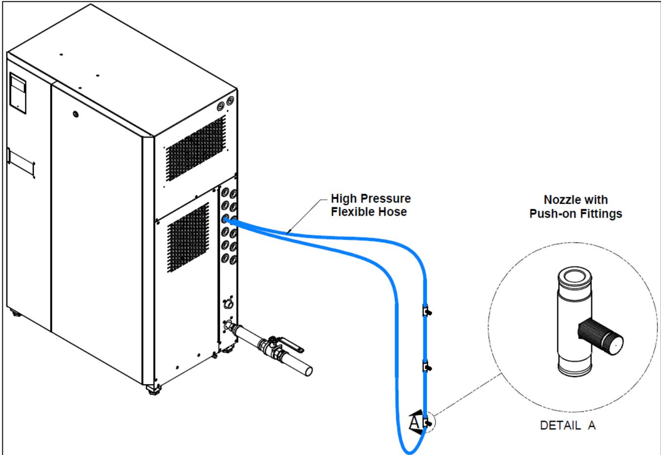
Illustration 19 - Typical Installation with Flexible Nylon Hose
