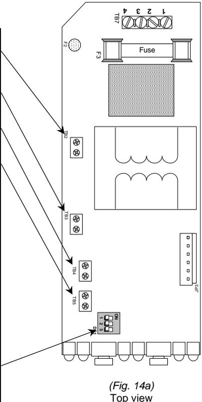
**10.2. P.C. Board for Modulating Humidifier**
