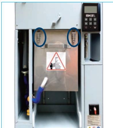
Disengage the 2 clamps
