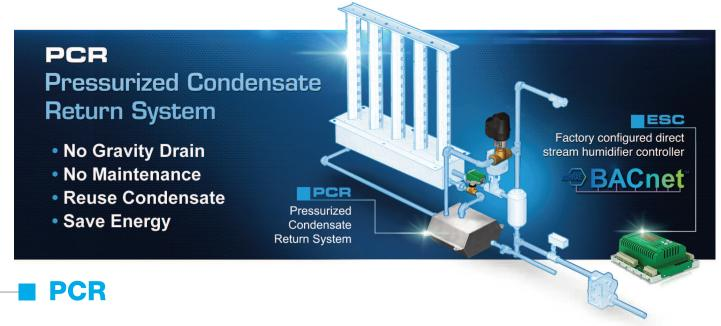
The Neptronic pressurized condensate return (PCR) system returns condensate generated within the steam dispersion tubes of a direct steam humidifier back to the steam source. Presently, the only other available technology is a pressurized steam humidifier with a heat exchanger (or re-evaporator).
